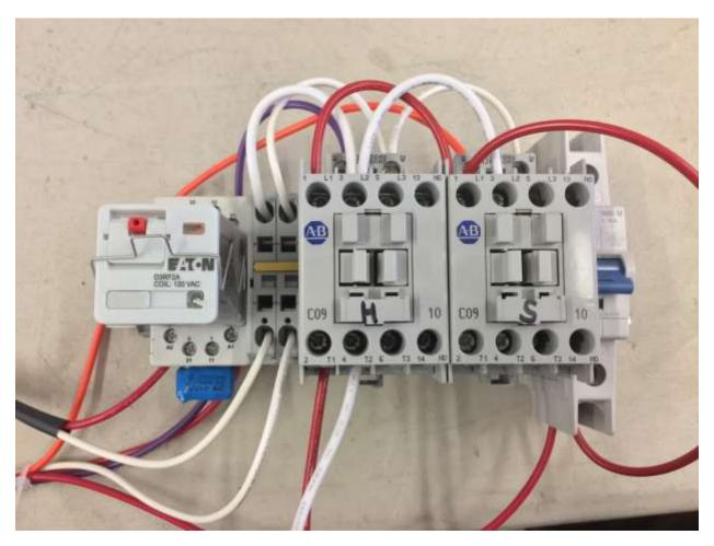
Thermal Overload Ice Cube Relay
