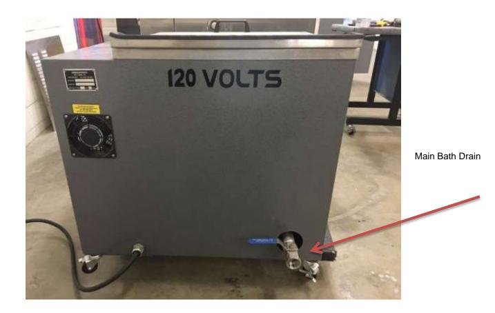
• Fill the wash tank with water (see note at the end of this section) and the proper dilution of soap until the machine is 2/3 full. Using hot water will shorten the amount of time required to reach the desired temperature. Check drain assembly to insure that there is no leakage.
