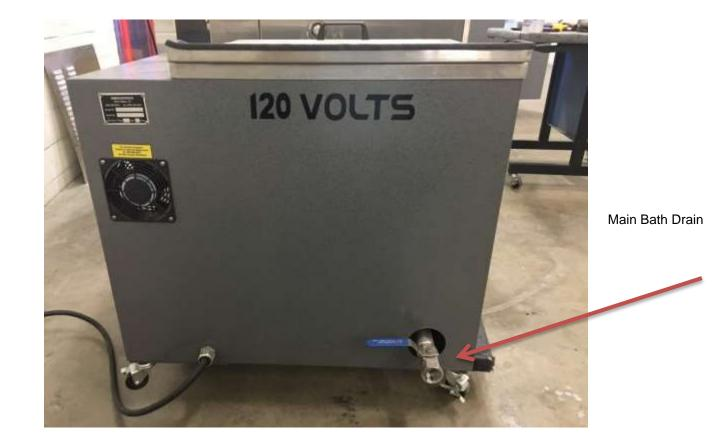
• Fill the wash tank with water (see note at the end of this section) and the proper dilution of soap until the machine is 2/3 full. Using hot water will shorten the amount of time required to reach the desired temperature. Check drain assembly to insure that there is no leakage.
