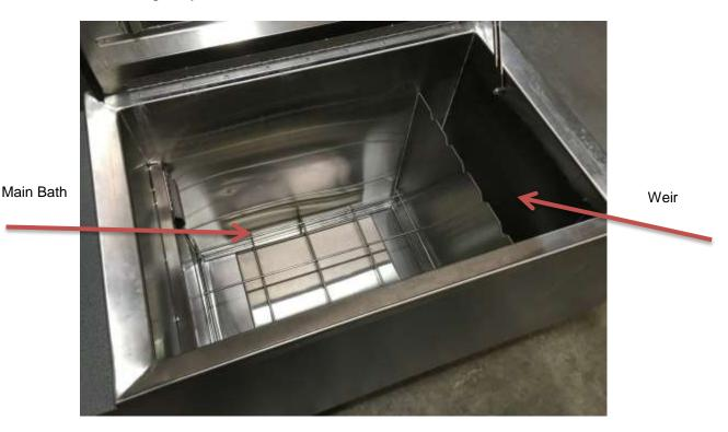
• If either the weir or machine tank do not have enough water the pump will be damaged and the machine will fail. Once the proper amount of water has reached the low level sensor, just below the spray bar, it will be activated allowing the machine to function properly.
