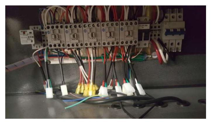
Float Sensor Ice Cube Relay Power Contactor Heat Contactor Sonics Contactor H
