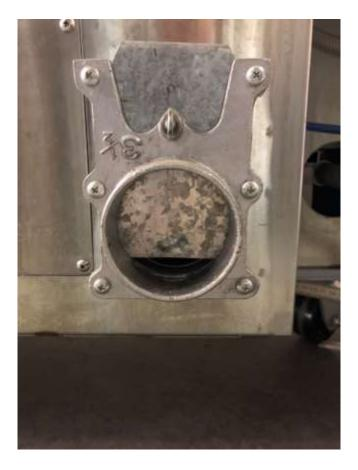
There is also an exhaust damper located on the rear of the console. This is to expel the humidity laden moist air. The dryer dries by moving a large volume of dry air over the items to be dried. The dryer is <u>not</u> an oven. An oven dryer would likely use temperatures in excess of 212° F that would likely boil off the water and may leave water mark residue.
