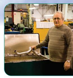
Manufacturing Engineer Bud Greener loads a precision-bent tube into an Omegasonics ultrasonic cleaning system.
