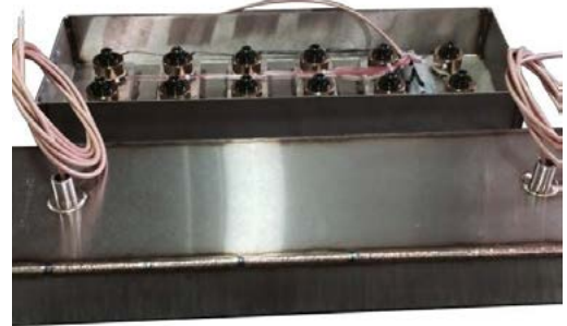
(Fig. 2) Two Ultrasonic Transducers: with the lid off (back), with the lid welded on (front)
