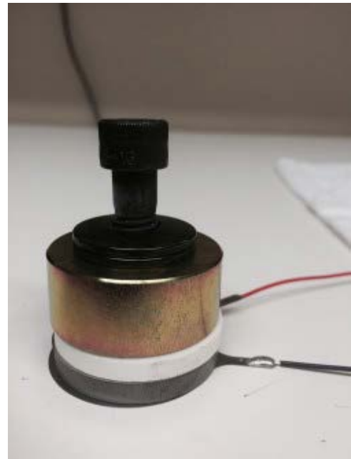
(Fig. 4) Piezoelectric Transducer Parts Assembled
