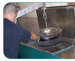
After a two-minute cleaning cycle, the stack is lifted out of the Omegasonics and tilted to drain water from between the blades.
