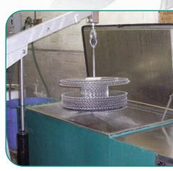
Dirty blades go into the Omegasonics PowerPro 6000, still carefully stacked as they were during transport to the shop.
