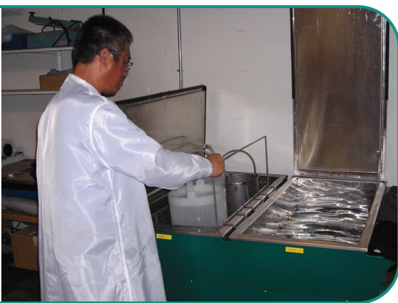
Parts are placed into the primary ultrasonic cleaning bath.
