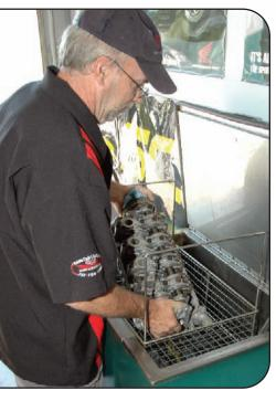
A four-stack carburetor requires very little teardown before it is ready for its deep cleaning in the Omegasonics Pro Plus.
