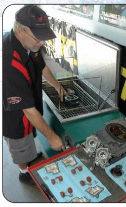
The Omegasonics Pro Plus handles all types of motorsports engine components.
