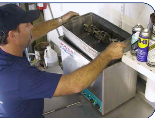
Multiple carburetors can be cleaned at the same time with the Omegasonics 4775.
