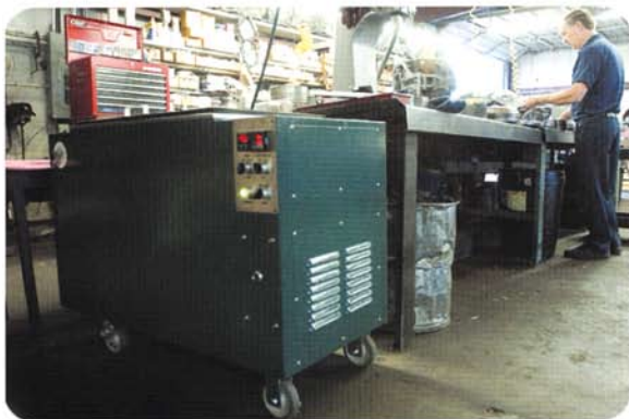
Ultrasonic cleaning machines come in a variety of sizes, many small enough to sit directly on or adjacent to a workbench, making them convenient to use.
