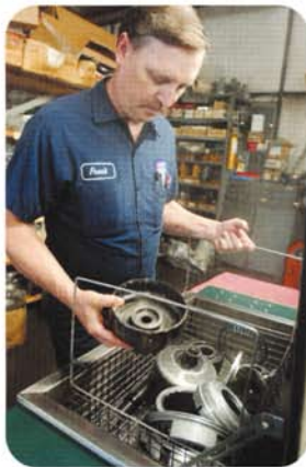
Cleaning transmission parts ultrasonically gets them as clean as or cleaner than conventional spray washers, their manufacturers say, and the ultrasonic action is perfect for small parts with intricate crevices, as in valve bodies.
