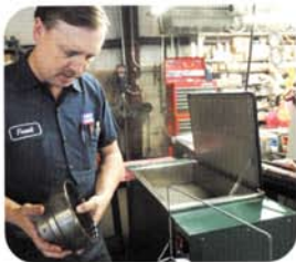
Cleaning transmission components in an ultrasonic machine is as simple as loading the parts into a washer basket, closing the lid and pushing a button.
